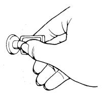
To lock or unlock the freezer you must hold the key in the lock while turning. The lock is spring loaded so the key cannot be left in the lock.
